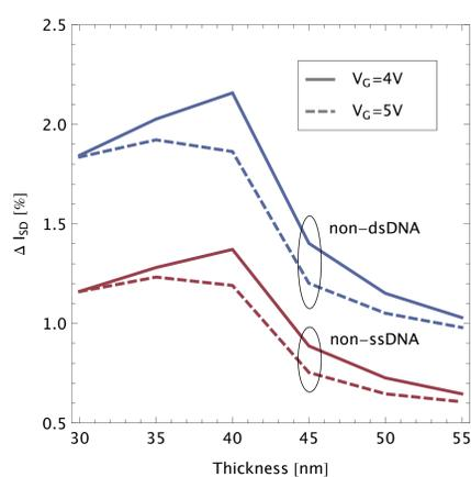
Fig. 5: Current change as a function of the nanowire thickness.
