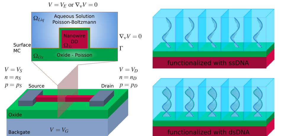
Fig. 1. Left: schematic cross section of the nanowire biosensor. The silicon nanowire is described by the drift-diffusion model, while the interface and the surface layer in the electrolyte are modeled by a Monte-Carlo approach. Boundary conditions are also indicated. Right: a nanowire functionalized with ssDNA as probes without any target molecules (top) and a nanowire functionalized with ssDNA with a target ssDNA strand (dsDNA, bottom).
